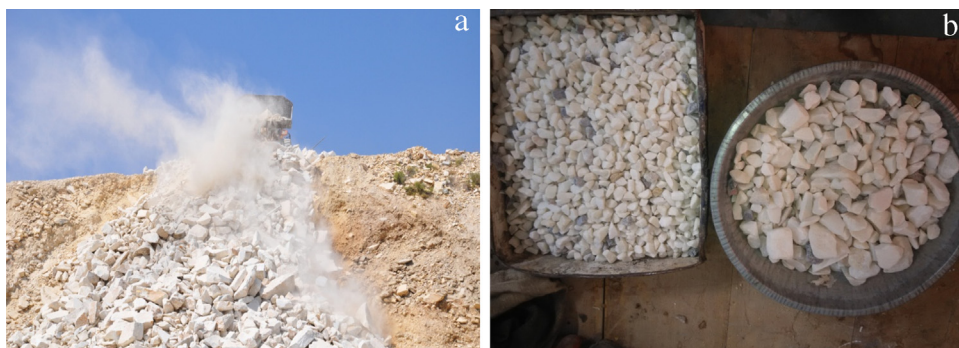
Fig. 1. (a) Marble waste dumped on site (b) Coarse aggregates from marble waste.
