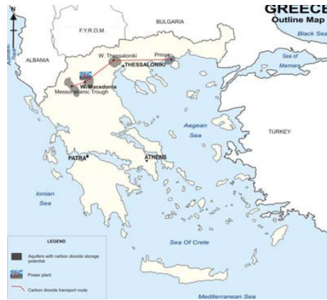
Figure 1 Proposed pipeline route from the new capture-ready 650 MWe coal fired power plant to the candidate saline formations
