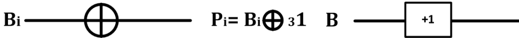
Fig. 6: (a) Illustration of a ternary Not gate; (b) Equivalent elementary gate realization
