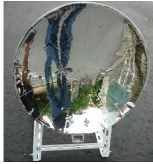
Fig.5 Parabolic solar collector
