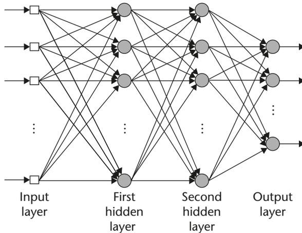
**Fig. 2.** Structural graph of multilayer perceptron (MLP) neural network model.
