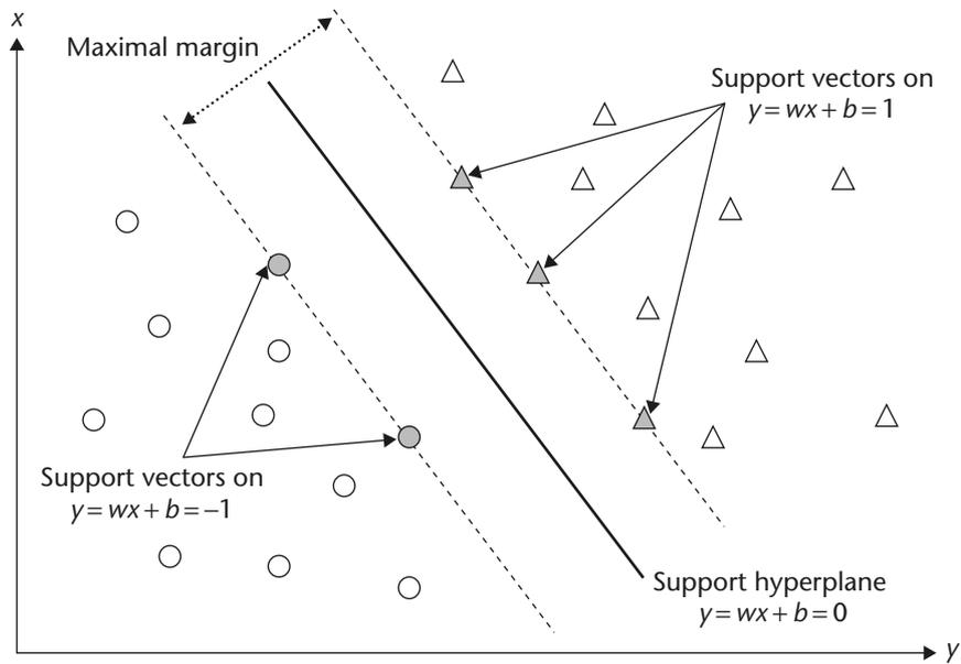
**Fig. 3.** An example of the optimal separating hyperplane of support vector machine (SVM) with the maximal margin between two parallel hyperplanes.
