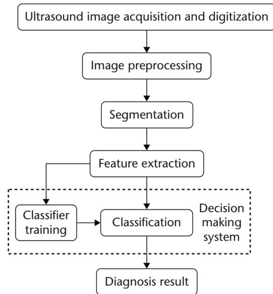
**Fig. 1.** Block diagram of a general computer-aided diagnosis (CAD) system for ultrasound imaging.
