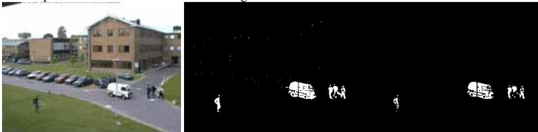
Figure 3 Original frame 399, frame 399 after background subtraction and after updated background subtraction frame 399
