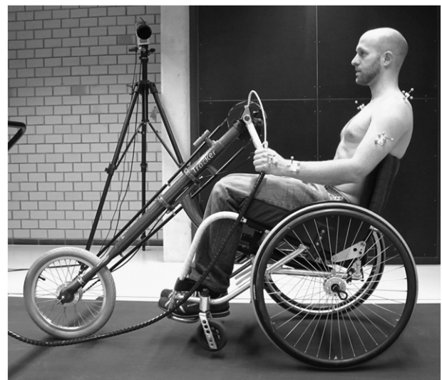
Fig. 1. Subject sitting in the instrumented handbike with cluster markers attached to the thorax, acromion, upper arm, lower arm and hand.
