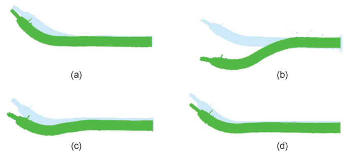
Figure 12. Deformation of the distal after 15 s moving with light blue color at t = 0 s and green color at t = 15 s. (a) Direct mapping with highest stiffness; (b) direct mapping with minimal movements [ \alpha = 1; \beta = 25 ]; (c) direct mapping with minimal movements [ \alpha = 10; \beta = 1 ]; (d) incremental mode with highest stiffness.
