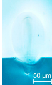
Fig. 7. Cross section of a welding seam in D263 under the following conditions NA = 0.55 , P = 6 W, v = 30 mm/s, f = 1 MHz
