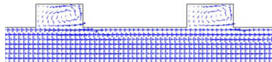
Fig.4 Velocity Vector of Flow Field at Bionic Ring Grooves Part of Bionic Nozzle
