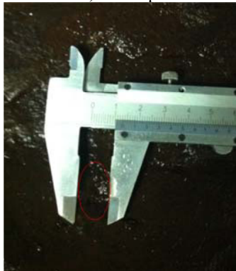
Fig.6 The Crushed Pit on Oil Shale Sample Caused by Ordinary Nozzle
