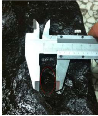
Fig.7 The Crushed Pit on the Same Oil Shale Sample Caused by Bionic Nozzle
