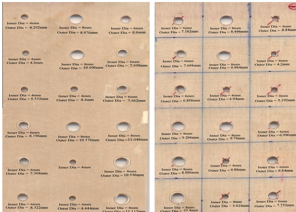
Figure 3 Top and bottom surface of drilled specimen with dimensions.
