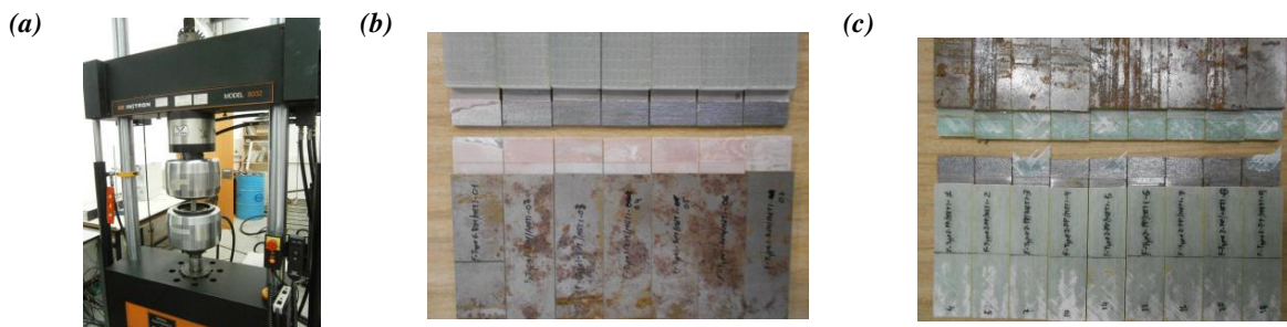
Fig. 8. (a) Fatigue testing equipment; (b) adhesive bonding specimens after fatigue testing; (c) pre-preg specimens after fatigue testing.
