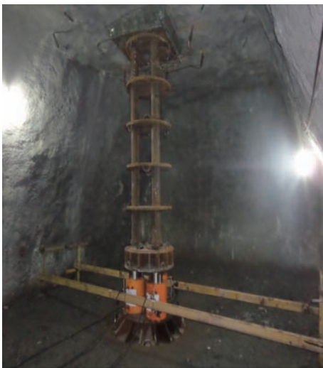
Fig. 2. Testing device for a tunnel compression test (Cihaxia).
