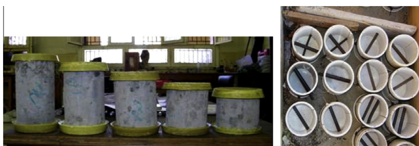
Figure 5 Non-standard molded reinforced cylinders comparable to extracted cores.
