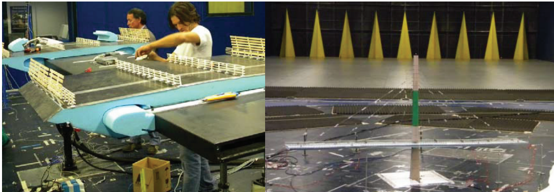
Figure 4: Wind Tunnel Testing: deck section and balanced cantilever from Central Tower
