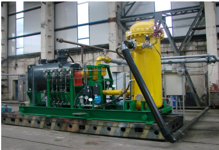
Fig. 2. Helicoidally expander - generator system - isometric view [2].
