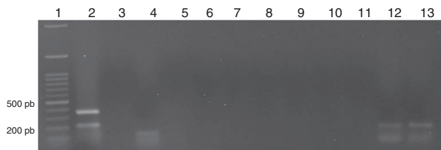
Figure 1 Representative image of a patient with LAL. Lane 1: Molecular weight marker; Lane 2: \beta -2-microglobulin (394 pb) and GAPDH (221 pb); Lane 3: BCR-ABL M (–); Lane 4: BCR-ABL m (150 pb); Lane 5: E2A-PBX1 (–); Lane 6: TEL-AML1 (–); Lane 7: AF4-MLL1 (–); Lane 8: PML-RAR \alpha (–); Lane 9: AML1-ETO (–); Lane 10: MAGE-A3 (–); Lane 11: NY-ESO1 (–); Lane 12: ABC-B1 (201 pb); Lane 13: ABC-G2 (206 pb).
