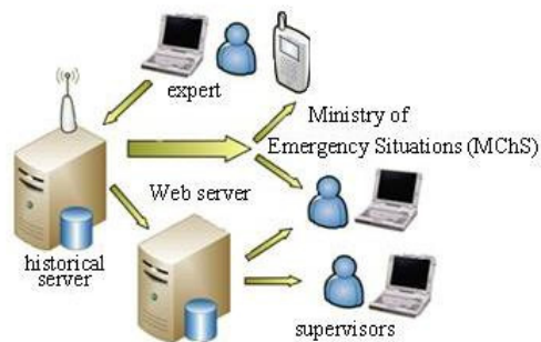
Fig. 3. Structure of small concrete bridge monitoring system
