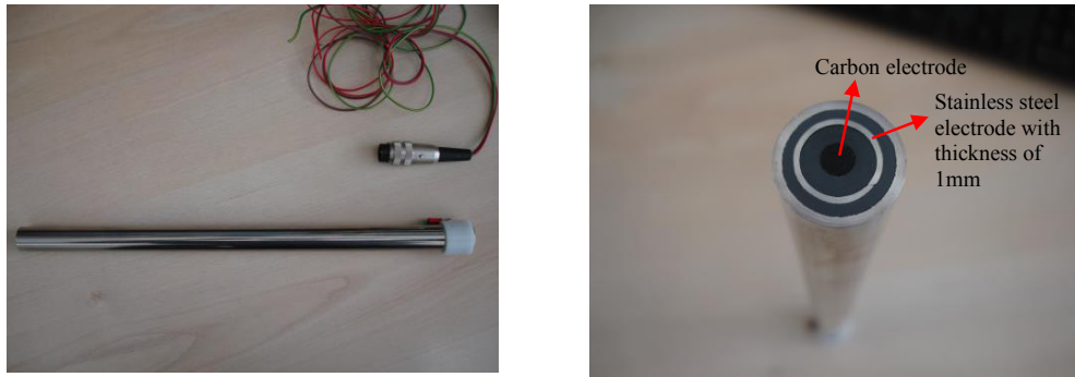
Fig. 1. photographs of the probe with two-electrode sensor.
