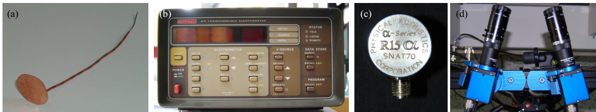
Fig. 3. (a) Typical electrode and (b) electrometer Keithley, 6517A used for the PSC technique; (c) typical R15 \alpha acoustic emission sensor; (d) the two cameras of the digital image correlation technique.
