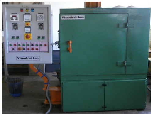
Fig. 2.(a) Biaxial Rotational Moulding Machine;
