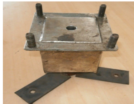
(b)Stainless Steel Hollow Mould
