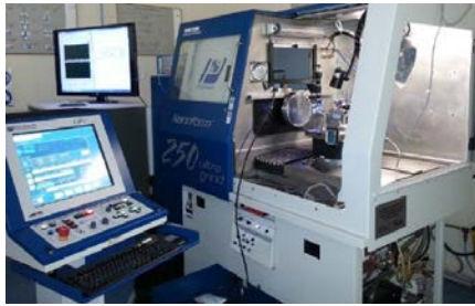
Fig. 1. Precitech Nanoform 250 Ultra-high precision lathe
