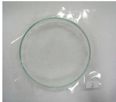
Fig 1. Test dish used for measuring WVTR by the gravimetric water method of ASTM-E96/E96-05 Standard
