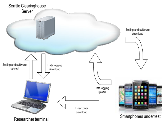
Fig.4. The proposed cloud-based architecture
