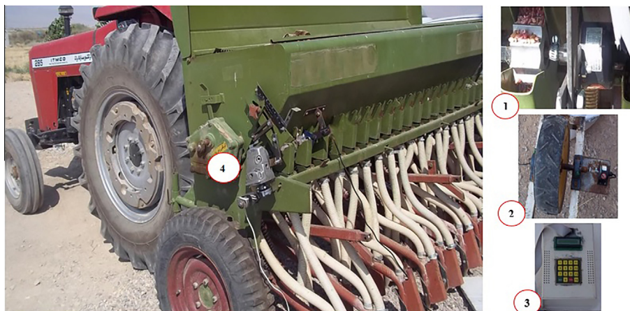
Fig. 4 – Equipped grain drill with new FSMU (1-digital encoder of seed metering shaft, 2-digital encoder of SGW, 3-control box via LCD and keyboard and 4-variable-rate DCM).
