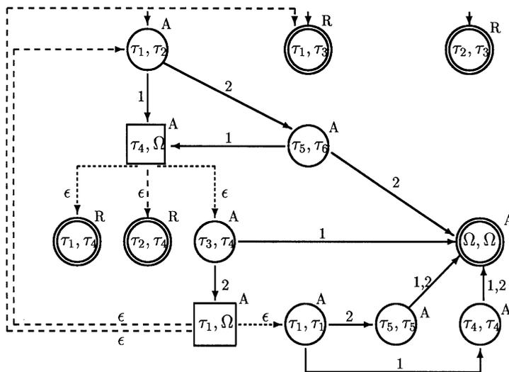
Here, we draw with a square the OR nodes and with a circle the AND nodes, and with a double circle the FINAL nodes. The “non-deterministic” edges outgoing from the OR nodes, are dashed. The initial nodes are denoted by an incoming arrow.
