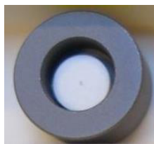
Fig. 1. Sample with tablet of \text{Na}_2\text{SO}_4 before testing.
