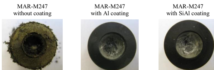
Fig. 4. Samples from MAR-M247 after 64 hours of testing.
