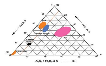
Fig.1 Composition of sludge, coal, clinker and raw material.
