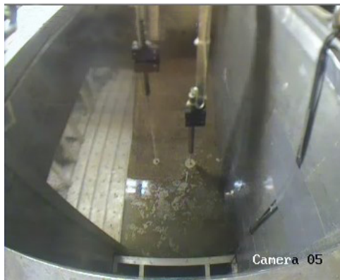
(b) Slope toe sliding at the normal water level.
