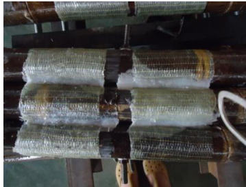
Fig. 7. Failure mode of bolted bamboo joint reinforce with FRP sheets.
