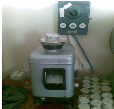
Fig. 1. (a) Measuring of heat conductivity of soil by device "MIT 1"; (b) determination of soil humidity by the method of drying to permanent mass
