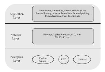
Fig. 1. Architecture of IoT
