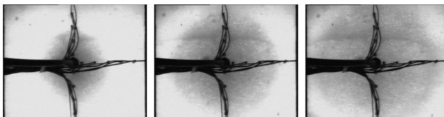
Fig. 4. Forced drainage experiments in parabolic flights: picture of a foam at three different times, evidencing isotropic diffusion. The liquid is injected at the centre, the wires are connections to electrodes; note that the wetter foam appears dark. Adapted from ref. [20].
