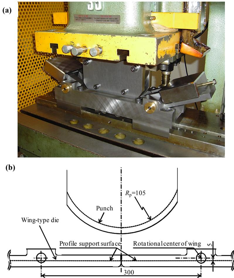
Fig. 2. Press bending setup. (a) Appearance of bending die at lower dead point and (b) main parts and dimensions of tooling.
