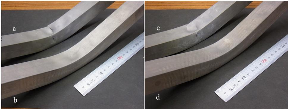
Fig. 4. Appearance of specimens after press bending. (a) TP350 without axial tension, (b) TP350 stretch bending, (c) TP450 without axial tension and (d) TP450 stretch bending.
