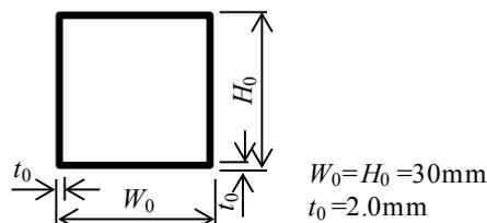
Fig. 1. Cross-sectional shape and dimensions of square tube.
