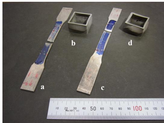
Fig. 3. Appearance of specimens after tests. (a) TP350 tension, (b) TP350 compression. (c) TP450 tension and (d) TP450 compression.
