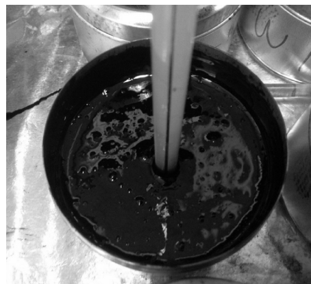
Fig. 5 – Foaming observed during the test.
