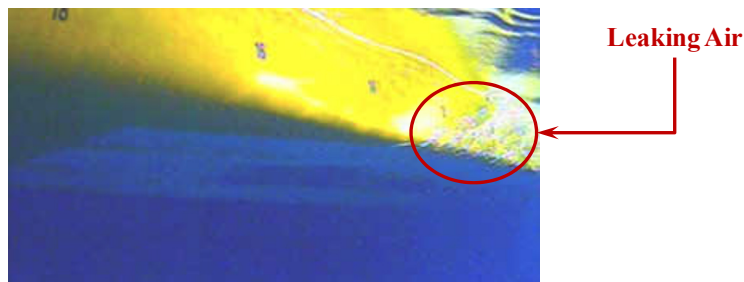
Fig. 16 Captured air layer at V_S = 14.5knots in the air injection condition I-B.
