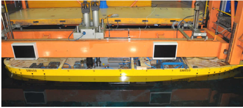
Fig. 14 Model ship prepared for the resistance test in the towing tank.
