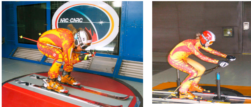
Fig. 1 (a) skier in full tuck position at NRC wind tunnel; (b) skier in upright position at GMAL wind tunnel
