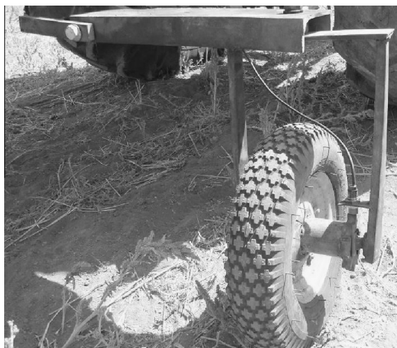
Figure 2 The fifth wheel for measuring the real forward velocity.
