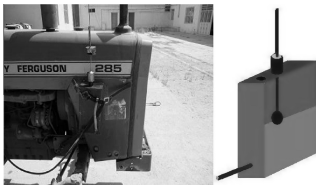
Figure 1 Fuel meter to measure the fuel consumption.
