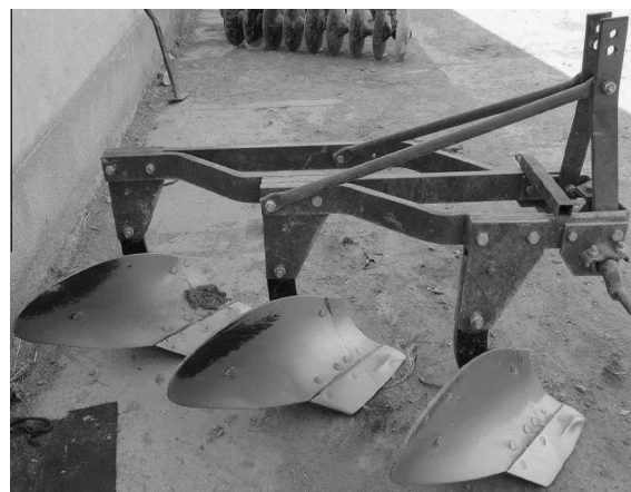
Figure 3 The moldboard plow with three furrows.
