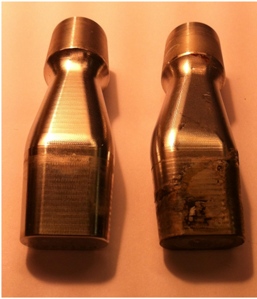
Fig. 7. Significant damage to the surface of the retrieved cone (right) compared to an unused cone (left).
