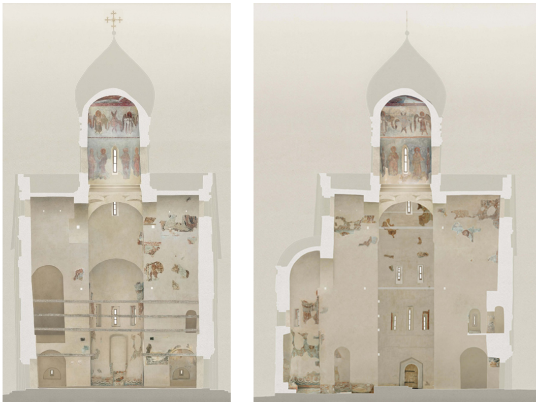
Fig. 2. (a) - The Eastern wall of the Church, preserved fragments of frescoes, (b) - The South wall of the Church, preserved fragments of frescoes
