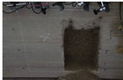
Fig. 6. Extraction of ore to form primary room.
