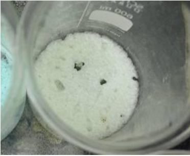
Fig 6. \text{Al}_2(\text{SO}_4)_3 \cdot 5 \text{H}_2\text{O} produced from computer PCB
