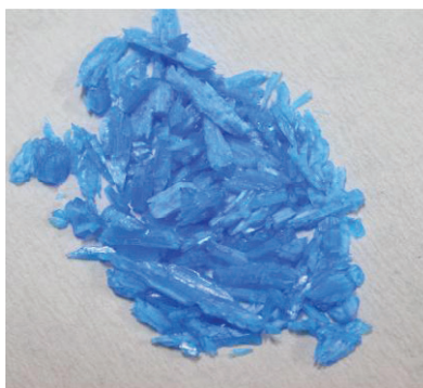
Fig 5. CuSO 4 .5H 2 O crystals produced
