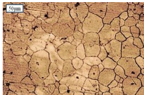
Figure 10 Microstructure of Base material AZ31B-O Mg alloy at 200X
