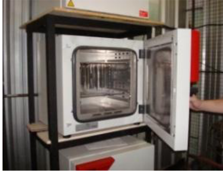
Fig. 2. Oven with air forced recirculation.
