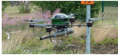
Fig. 1. Micro-drone equipped with gas-sensitive payload in flight.
