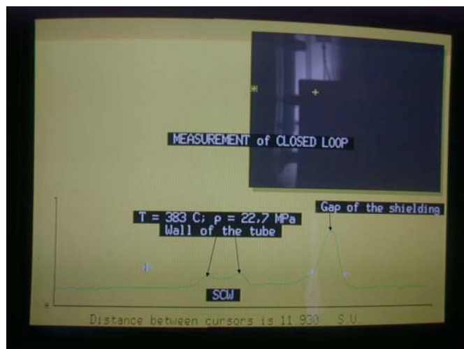
Fig. 8. The light intensity between the yellow crosses shown Fig. 7. on SCW state
