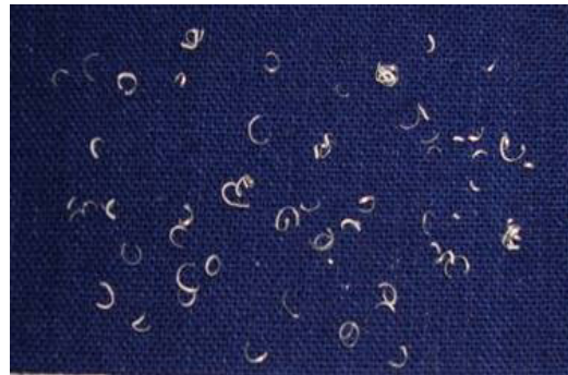
Fig.6. Chip formation at optimal parameters (150m/min, 0.05 mm/rev and 0.5mm DoC)
