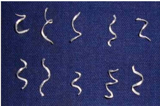
Fig.5. Chip formation at initial parameters (100m/min, 0.05 mm/rev and 0.5mm DoC)
