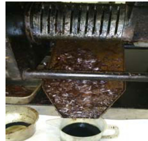
Fig. 3 Mechanical oil extraction through a screw press
