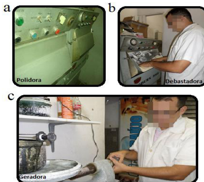
Fig. 6. (a) Polishing machine; (b) Planning machine; (c) Lens generator machine.
