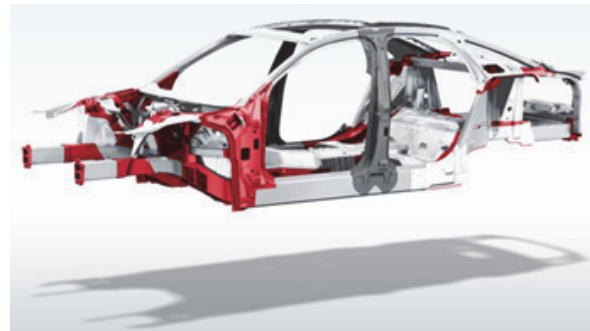
Fig.2 Audi Space Frame (ASF) [5]: chassis of an Audi A8 manufactured with magnesium and aluminium elements manually welded because of the defectiveness of the melting process
